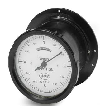
The **IM120A** the case contains a magslip receiver which is energised by 50 volts AC and accepts signals from the transmit magslip in the form of a synchronous link. Therefore, this receiver magslip follows the movement of the transmit magslip in the sensors indicating the direction of the wind. The position of the pointer on the magslip spindle is factory set and needs no further adjustment when installed. COMPATIBLE WITH THE IM146 ONLY
